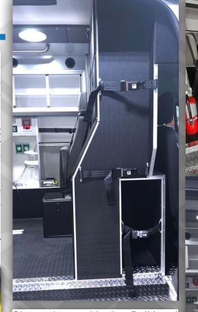
Shown here with the Bulkhead Doors option, There is still ample storage room. The center cabinet below the window extends to the area behind the attendant seat to allow for even more storage space.
